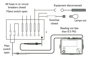
Note: Insulation testing must only be undertaken on de-energised circuits.
